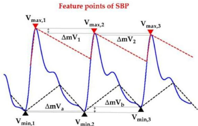
**Fig. 1:** Peak and valley detection algorithm for pressure pulse wave (PPW) signals.<sup>21</sup>
